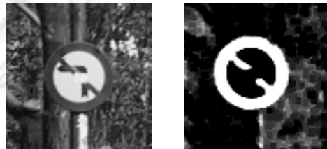
Figure 1: Left: RGB image of a road sign. Right: greyscale image where red pixels belonging to the border have been enhanced.
