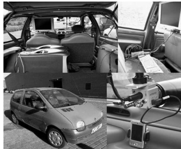
Figure 11: From left to right: CPU's where ADAS algorithms run. Keyboard and control screen. Experimental platform IVVI. Color camera, GPS and PDA.
