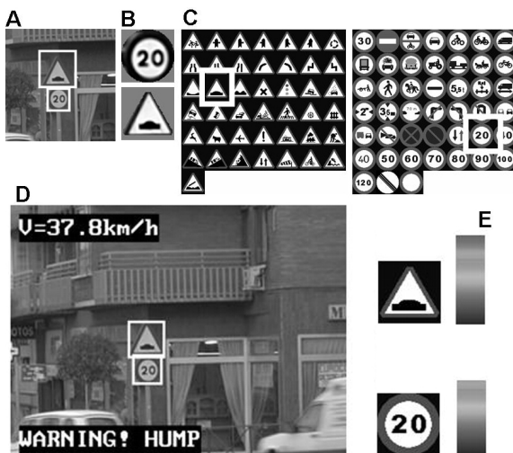
Figure 7: Recognition and Warning Stages. A) Detected road signs. B) Candidates to road signs. C) Recognition over the template. D) Output of the RSR system: shows the road image, the recognized road signs and E) its reliability level.
