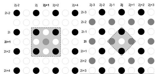
Figure 1: The two step NEDI interpolation. Original  $N \times N$  pixel are placed in a  $2N-1 \times 2N-1$  grid. Pixels at odd positions  $(2i+1, 2j+1)$  are then filled with the NEDI method (left) as weighted sums of the 4 diagonal neighbors. The remaining empty pixels are then filled in the same way after a  $45^\circ$  rotation of the grid.
