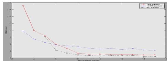
Figure 3: Rotation error varying with the number of lines.
