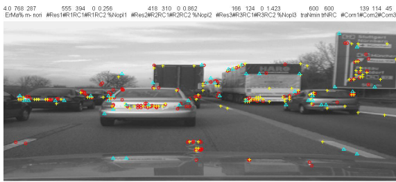
Figure 6: Corner candidates from two rotated ‘diagonal tests’ on three pyramid levels (centers not adjusted): ‘o’ = level 0, ‘+’ = level 1, triangles = level 2. The number of corner candidates is down to about 1/3 by the 2 nd test.
