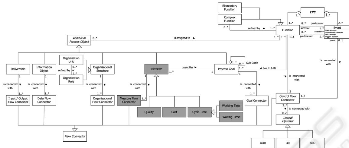
Figure 4: Extended EPC metamodel with performance measures.
