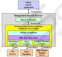
Figure 5: Implementation of an integrated search server based on IBM WebSphere Information Integrator OmniFind search engine.
