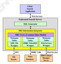
Figure 3: Implementation of a federated search server based on IBM DB2 Information Integrator and wrapper technologies.
