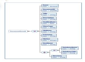
Figure 2: Schema of the common data model used to represent a search result.
