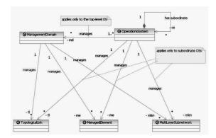
Figure 1: MTOSI model for Managed Domain.
