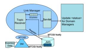
Figure 5: Asynchronous notification system for changes in the inventory data.
