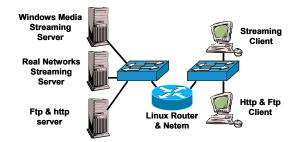
Figure 2: Testbed for the evaluation of streaming services performance on constrained variable user access lines.
