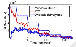
Figure 5: Windows Media streaming session and FTP delivery rate when bit rate decreases down to 350Kbps.
