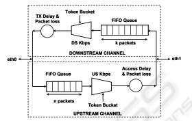
Figure 1: Model of the user access line implemented using a linux router, 2FastEthernet cards and *Netem*.
