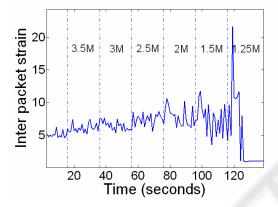
Figure 7: Inter-packet strain for a 1Mbps UDP flow and different DS rates (Mbps).
