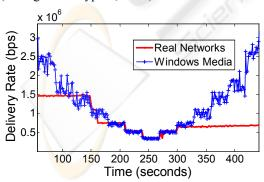
Figure 3: Delivery rate for Windows Media and Real Networks when access line conditions change.
