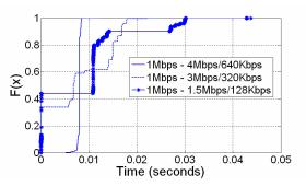
Figure 6: CDF of packet inter arrival time for different access line conditions.
