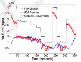
Figure 8: UDP streaming based on packet strain delivery rate estimation.
