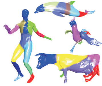
Figure 3: Results of the clustering process: dance with 14, dolphin with 9, chicken with 10 and cow with 6 clusters. Each cluster is colored differently and encoded separately.
