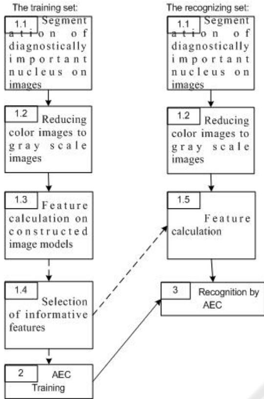
Figure 4: The descriptive scheme of recognition.
