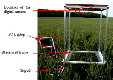
Figure 2: In Field image acquisition system.
