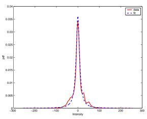
Figure 6: Histogram of the intensity differences collected from 19 images. The obtained distribution is well approximated by the best fit SEF (3) with parameters  $\alpha = 0.02$  and s = 9.
