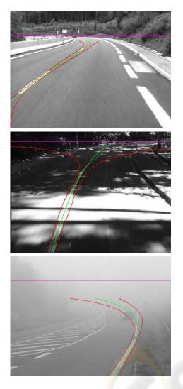
Figure 7: Three examples of detected lane-marking of degree 3 (in green). The uncertainty about the lane-marking location are also shown (in red).
