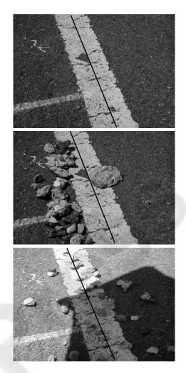
Figure 3: Three of the 150 images of the same marking with different perturbations. The black straight line shows the reference marking position.
