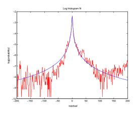
Figure 4: Log histogram of the residual errors in feature centers collected from 150 images after local marking extraction. The obtained distribution is well approximated by the best fit SEF (3) with parameters  $\alpha = 0.05$  and s = 1.1.
