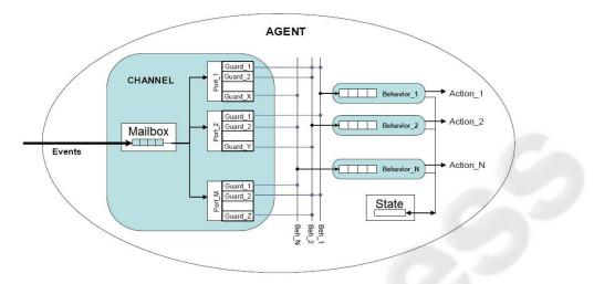
Fig. 4. BESA-ME agent level model. The boxes represent the data structures of the agent.
