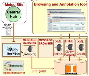
Figure 2: Architecture of the system.
