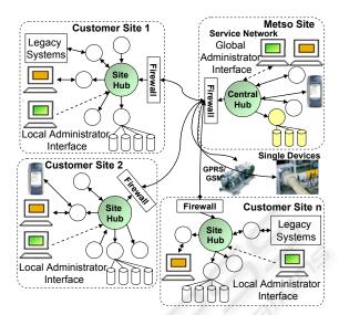
Figure 1: Site Hub network architecture.
