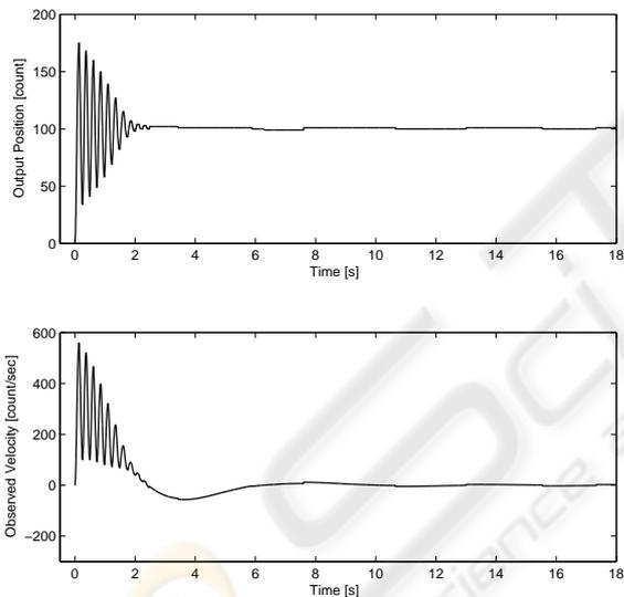
Figure 11: Experimental results employing the observer from Theorem 2.
