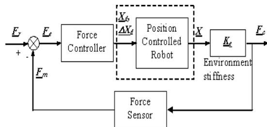
Figure 1: Robot force control.
