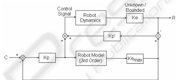
Figure 4: Robust force controller.
