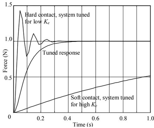
Figure 2: Effect of environmental stiffness.
