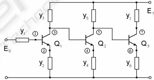
Figure 1: Circuit topology for three-cell transistor amplifier.
