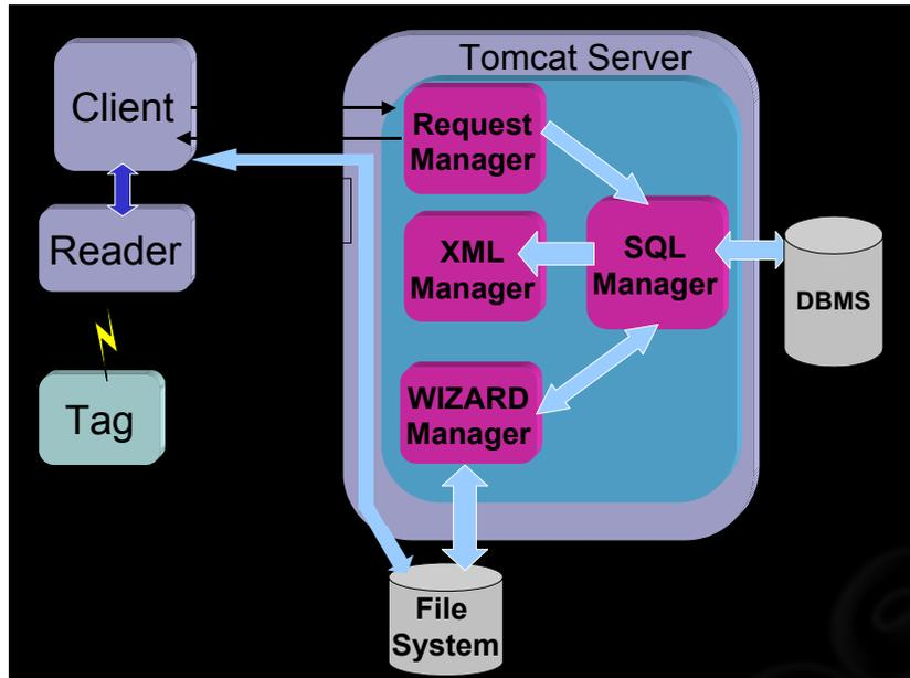
**Fig. 3.** Server architecture and interactions with the client.
