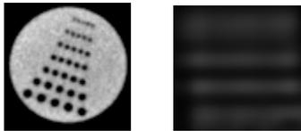
Figure 7: Details of a CT (left) and zoomed MRI image (right) showing the spots used for computing the high contrast spatial resolution. In the case of the MRI image the spots are not distinguishable.
