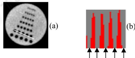
Figure 6: Locating reference points on a CT image of a resolution phantom, using the profile-based method. (a) Axial image of a resolution CT phantom (b) One-dimensional profile from the second row of air holes drilled in an epoxy resin-based insert of the CT phantom; the arrows point to locations of minima.
