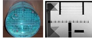
Figure 1: ACR phantom used for MRI QA (left), and a typical sagittal MRI image (right).
