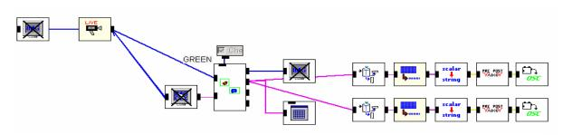
Figure 5: EyesWeb algorithm architecture for tracking a single color.
