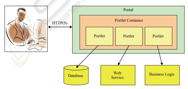
Figure 1: JSR 168 defines standard between portlets and portlet container.
