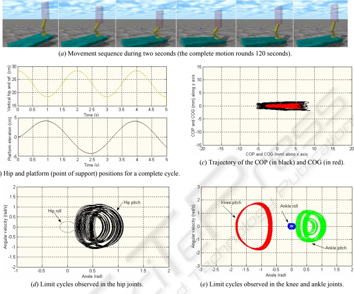
Figure 4: Simulation results obtained for the robot standing on inclined ground with variable slope.
