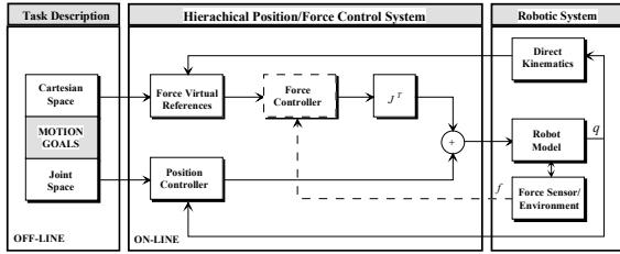
Figure 2: Blocks diagram of the hierarchical control scheme.
