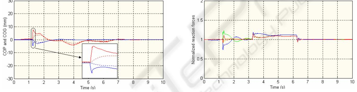
(c) Location of the COP (solid line) and projected COG (dotted line) along the x-axis (in red) and along y-axis (in blue). Normalized normal reaction forces at the corners of the foot: back right (in yellow), back left (in blue), front right (in green) and front left (in red).
