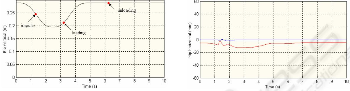
(b) Hip's vertical position under disturbances (left) and hip's horizontal position (right): along the x-axis (in red) and along the y-axis (in blue).
