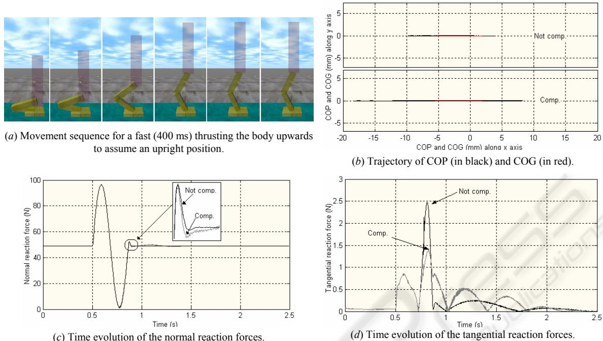
Figure 5: Simulation results obtained for the robot standing on level ground with the regulation of the tangential forces.
