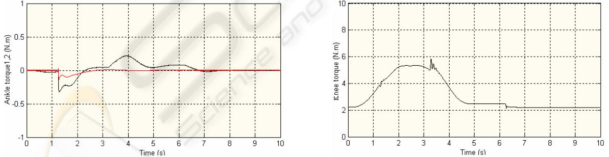
(d) Temporal evolution of the torques at the ankle joints (left) and knee joint (left).
