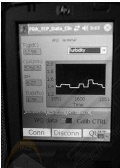
Figure 4: PDA interface for data visualization and remote calibration control.
