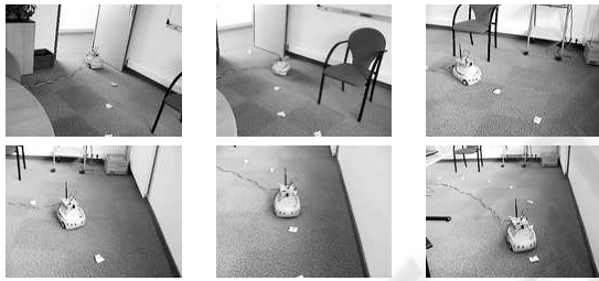
Figure 11: Following a visual route: the previously learnt visual path, about 10m long, is materialized on the ground. The pictures were taken during an autonomous run.
