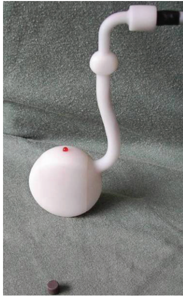
Fig. 7. Sensors support developed and the magnet used in the acquisition of the 3D mandibular movement.
