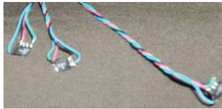
Fig. 2. Sensors used in our prototype system: AA002-02 from NVE Corporation.
