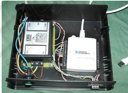
Fig. 8. Acquisition box with the DAQ and the power source used in our acquisition system.
