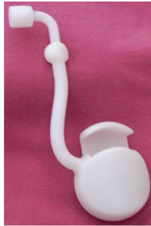
Fig. 5. The developed support for the sensors used materialized by rapid prototyping.
