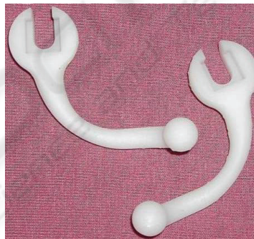
Fig. 4. Redesigned auricular pieces materialized by rapid prototyping.
