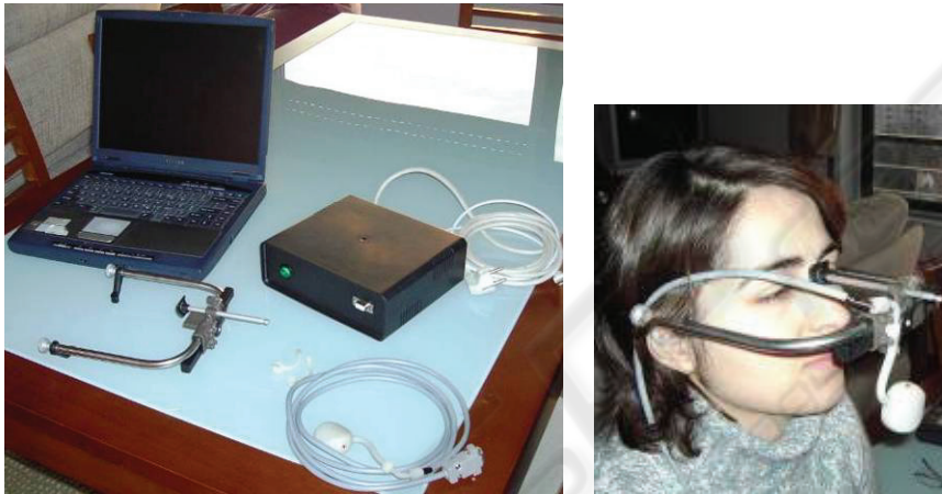
Fig. 14. Our prototype system for 3D mandibular movement acquisition and analysis and its usage.
