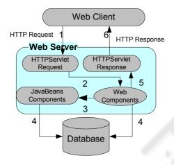
Figure 3.1: J2EE web application request handling
