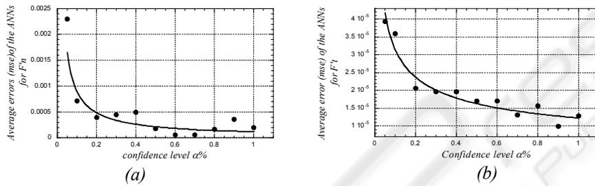
**Fig. 2.** Relation between the average  $\overline{MSE}$  errors of the 39 ANN structures and  $\alpha\%$ : (a)  $F'_n$  and (b)  $F'_t$
