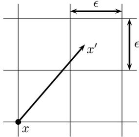
Figure 1: Simple grid of resolution  $\epsilon$ .  $V^i$  is known at the grid points, e.g. at  $x$ , whereas  $V^i(x')$  has to be interpolated
