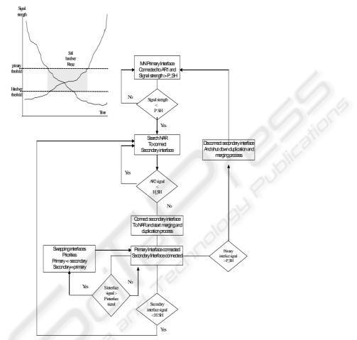
Figure 4, 5: Thresholds and Handover process
