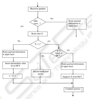
Figure3 : IPv6 flow merging algorithm
