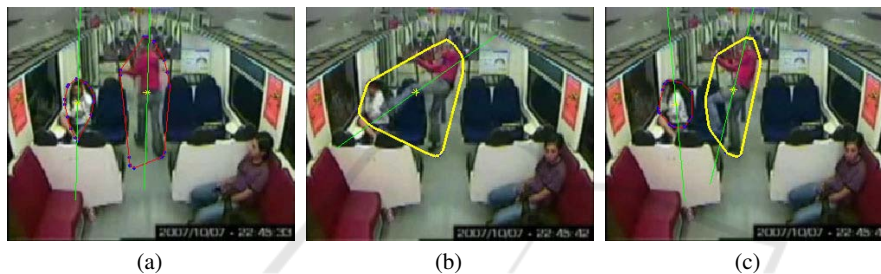
Fig. 8. Real scene in a public transport. In 8(a) two persons are detected. In 8(b) a sudden union between the two objects is found. A suspicious event keeps detecting in 8(c).
