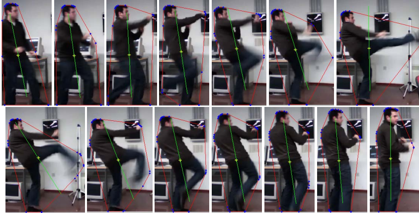
Fig. 5. Convex hull, centroid and principal axis of a person along several consecutive frames.
