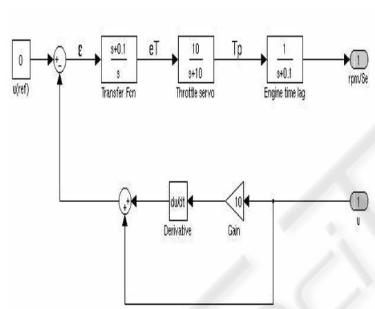
Figure 2: Velocity control system.
