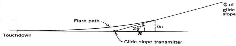
Figure 5: Geometry of the Glide Slope
