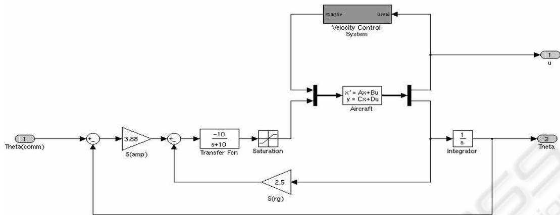
Figure 1: Basic autopilot block diagram
