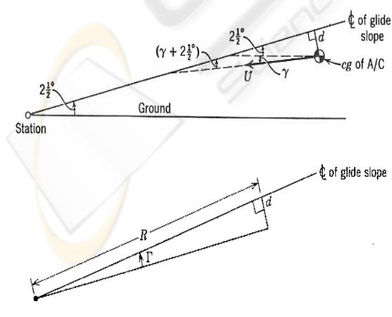
Figure 4: Geometry of Glide Slope Problem
