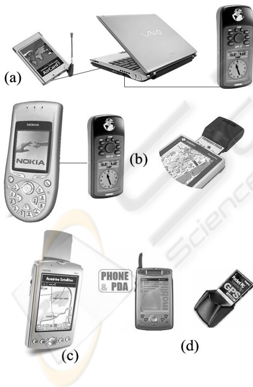
Figure 3: Candidate Hardware Configurations for Client Position Communication Device a) Compact PC with GPS receiver connected via GPRS Wireless PCMCIA card. b) PDAs with GPS. c) PDA with inbuilt GPS. d) PDA with GPRS and CF GPS
