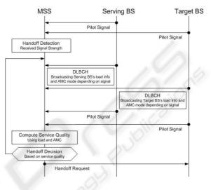
Figure 4: Smart handoff procedure
