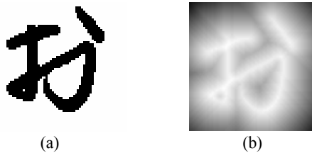
Figure 1:(a) Binarized pattern. (b) Distance transformation. (64x64 pixels.)
