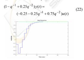
Figure 5: Open loop step response.
