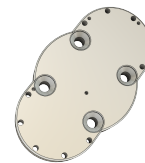
Figure 12: Central interface part connecting the two Rokubi sensors with the main sensor.
