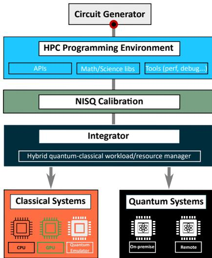
Figure 1: Heterogeneous software architecture for the integration of HPC and Quantum Computing resources.
