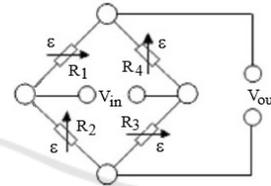
Figure 2: Wheatstone Bridge Circuit for Gauges Measuring Torsion.
