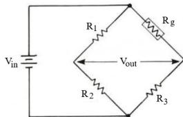
Figure 1: Simple Wheatstone Bridge Circuit.
