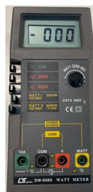
Figure 4: Lutron DW-6060 Watt Meter (School of Engineering, 2025).
