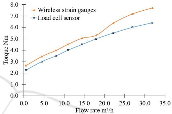
Figure 10: Shaft Torque versus Flow Rate.
