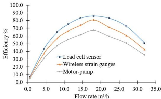
Figure 12: Efficiency versus Flow Rate.
