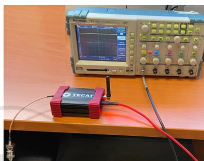
Figure 5: Connecting the Receiver and Oscilloscope for Laboratory Testing (School of Engineering, 2025).
