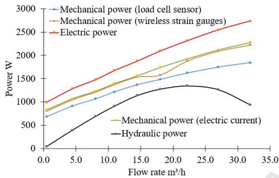
Figure 11: Power versus Flow Rate.
