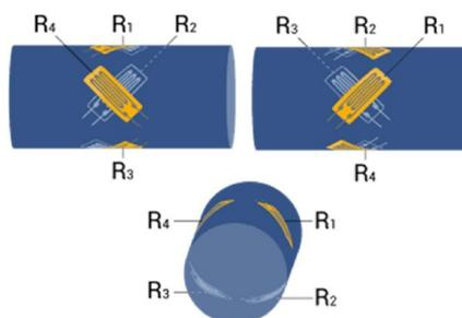
Figure 7: Arrangement of Strain Gauges on the Shaft (Hottinger Brüel and Kjaer, 2025).
