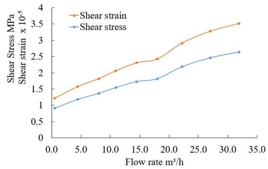
Figure 9: Shear Strain and Shear Stress versus Flow Rate.
