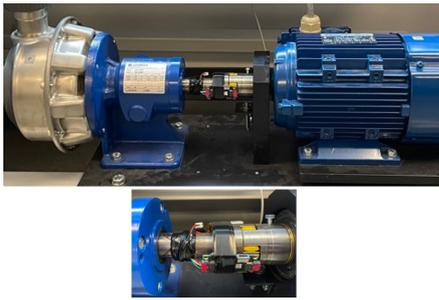
Figure 8: Strain Gauges on the Pump Shaft (School of Engineering, 2025).
