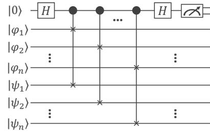
Figure 3: Solution sketch for the SWAP TEST pattern.
