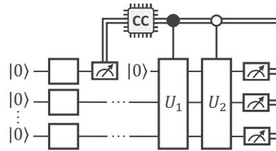
Figure 6: Overview of the solution sketch for the DYNAMIC CIRCUIT pattern.
