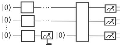
Figure 5: Overview of the solution sketch for the MID-CIRCUIT MEASUREMENT pattern.
