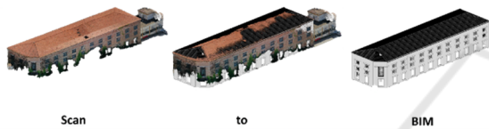
Figure 1: The 3D point cloud to the BIM model is achieved by importing the point cloud in .rep format into Autodesk Revit 2021 software.
