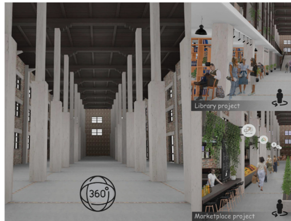
Figure 3: 3D online game environment. On the left, the building is obtained through the HBIM model import. On the right, two design proposals are created by users through the insertion of furniture elements imported by users and appropriately positioned in the scene.
