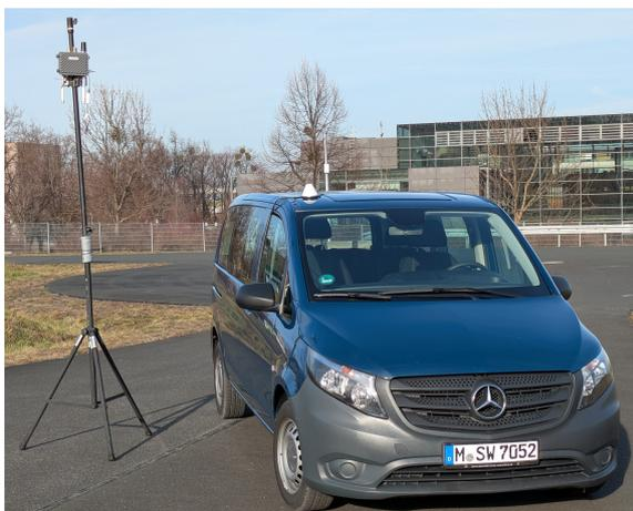
Figure 2: Measurement setup used for data gathering. On the left is the RSU mounted on a mobile tripod, on the right is the vehicle used for measurements. The V2X antenna is visible on the top of the car.
