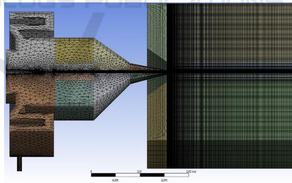
Figure 3: Meshed geometry model of the printhead and a free space area (Ungerer et al., 2023c).
