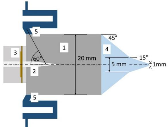
Figure 1: Schematic of the principle design of the AoD-jet printhead.
