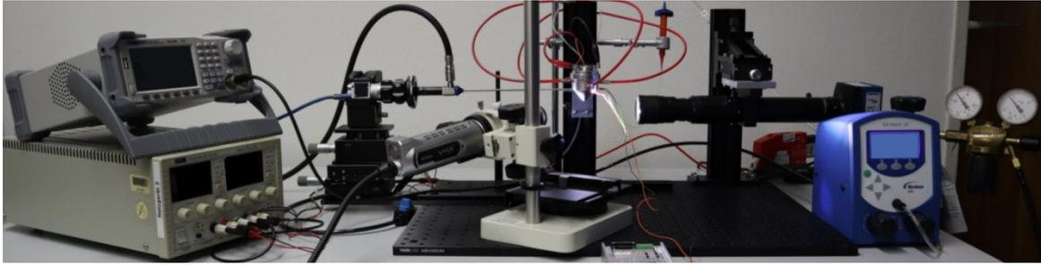
Figure 2: Laboratory setup of the AoD testbed.
