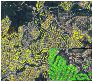
Figure 4: The image illustrates the PONNOT points (yellow) representing electrical infrastructure poles and their corresponding buffers (green), which simulate the coverage area of electrical infrastructure.
