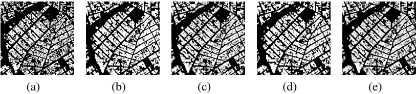
Figure 7: Prediction results for the Google Earth satellite image dataset. (a) Ground truth; (b) LinkNetB7 BCEIoU; (c) LinkNetB7 DICE BCE; (d) D-LinkNet50 BCEIoU; (e) D-LinkNet50 DICE BCE.
