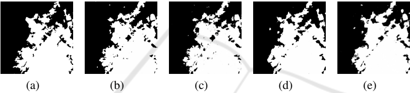
Figure 9: Prediction results for the Landsat 8 satellite image dataset. (a) Ground truth; (b) LinkNetB7 BCEIoU; (c) LinkNetB7 DICE BCE; (d) D-LinkNet50 BCEIoU; (e) D-LinkNet50 DICE BCE.
