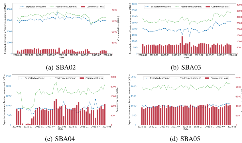
Figure 5: Historical series of feeder measurements, expected consumption, and NTL for the SBAU substation.
