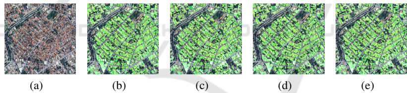
Figure 6: Prediction results overlaid on the original for the Google Earth satellite image. (a) Original image; (b) LinkNetB7 BCEIoU; (c) LinkNetB7 DICE BCE; (d) D-LinkNet50 BCEIoU; (e) D-LinkNet50 DICE BCE.
