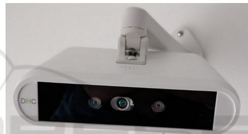
Figure 1: Sensor box from DHC mounted on a wall in the rooms.
