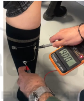
Figure 21: Electrical conductivity tests on textile.
