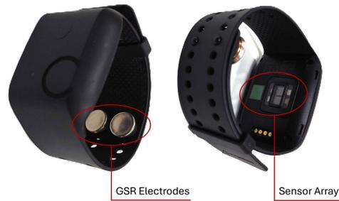
Figure 4: Empatica E4 wearable physiological measurement device.
