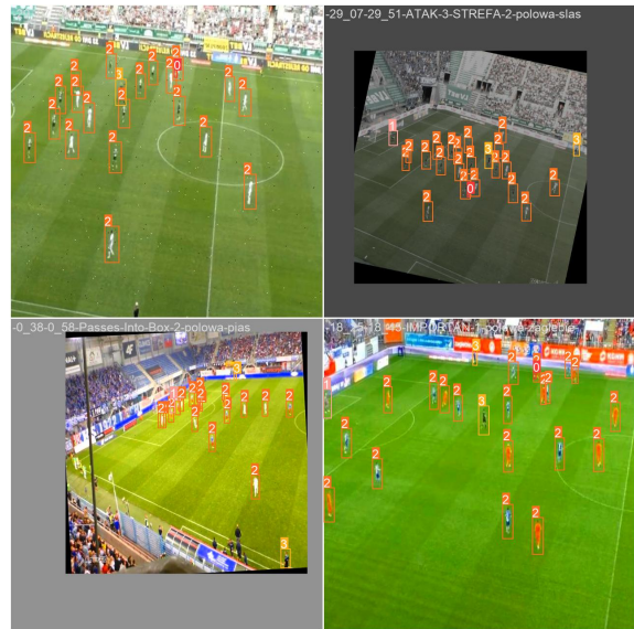
Figure 4: Examples of augmented frames from the dataset. Top left: noise, top right: rotation and blur, bottom left: rotation, bottom right: bounding box blur.
