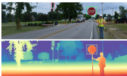
Figure 3: Depth-Anything V2: Obstacle detection on the road (Yang et al., 2024).
