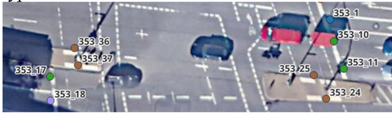
Figure 3: Visualization of geo data at intersection 353 – no of intersection as well as no of signal controller [maps.google.com].
