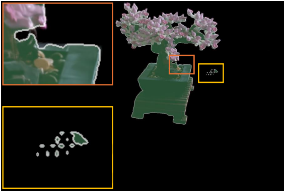
Figure 6: Example rendering overlaid with the corresponding mask. Yellow box: non-object pixels in mask are not reconstructed. Orange box: object pixels missing in mask are still reconstructed.
